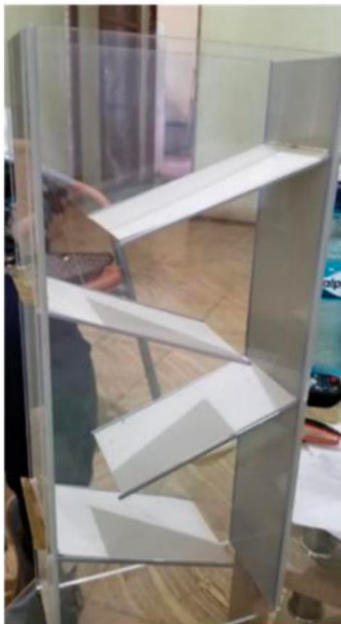
Figure 3 Silver-Covered Copper Plates in a ZigZag Arrangement
