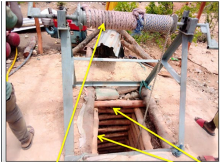
Absence of a wire winch rope
