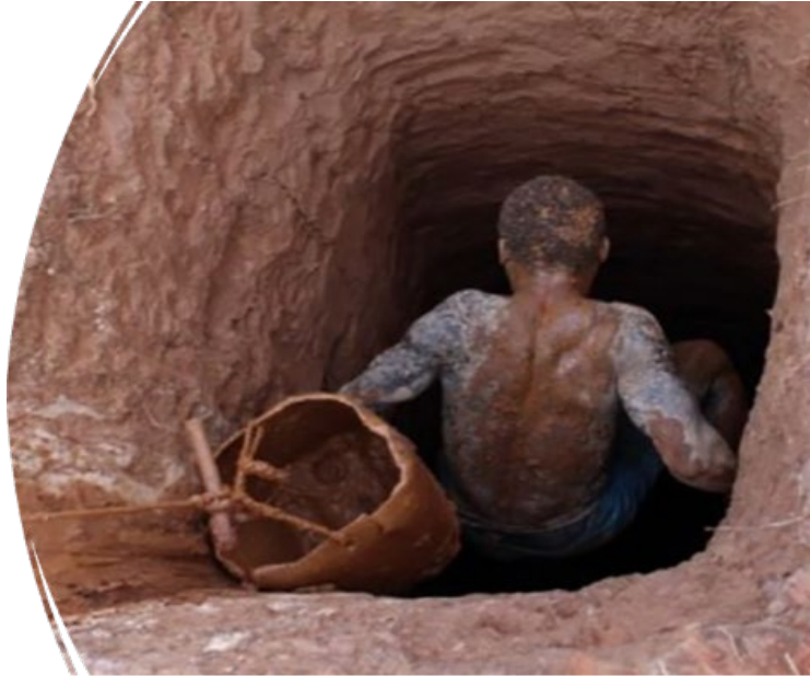
Absence of a wire winch rope
