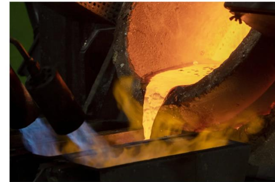
Melted gold flows out of a smelter into a bar mold at a plant run by the gold and silver refiner Argor-Heraeus in Mendrisio, Switzerland. Denis Balibouse/Reuters
