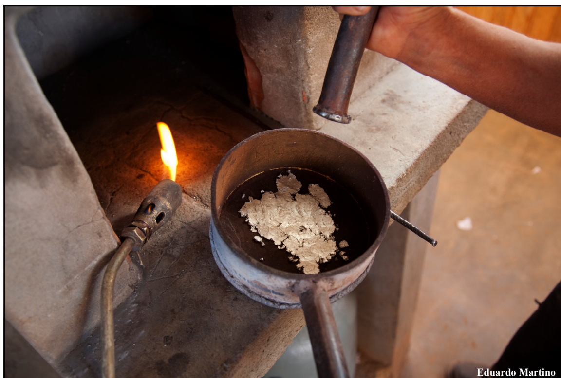
Heating the amalgam allows miners to obtain gold, but carries serious contamination risks
