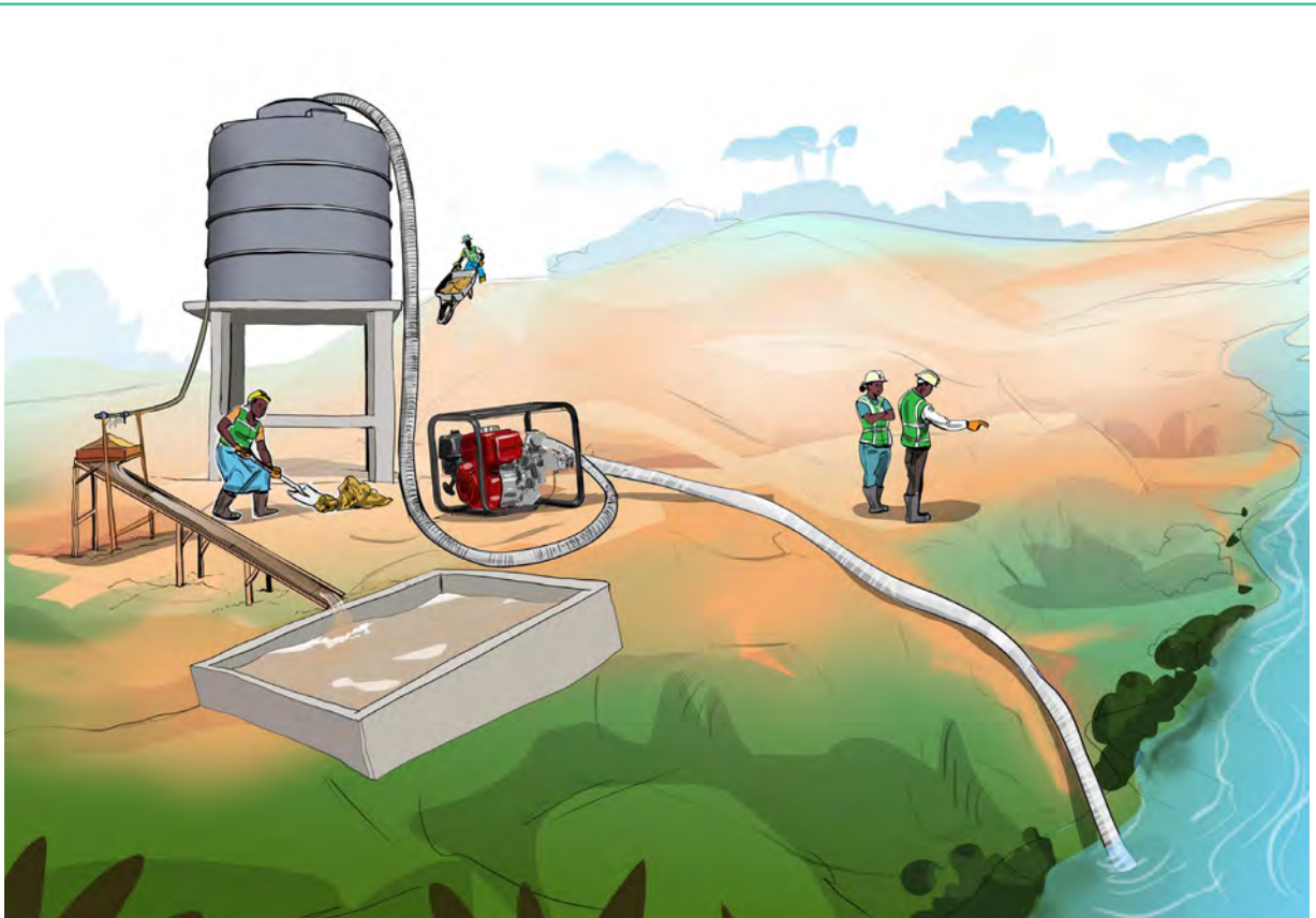
Image 31: Motor pump supplies process water for sluicing.
