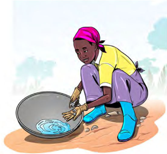
Image 5: Worst practice is whole ore amalgamation. Add mercury only to concentrates.
