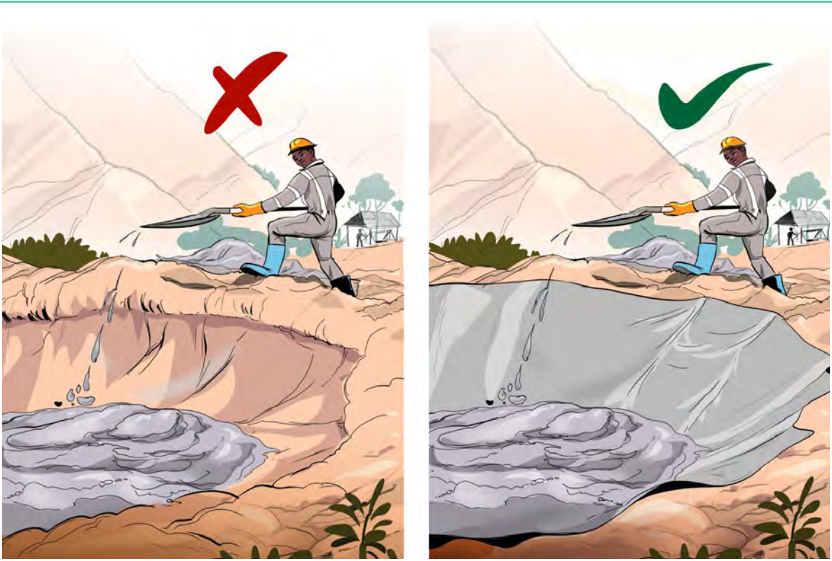
Image 3: Properly dispose of mercury-contaminated tailings by burying them in a lined pit.
