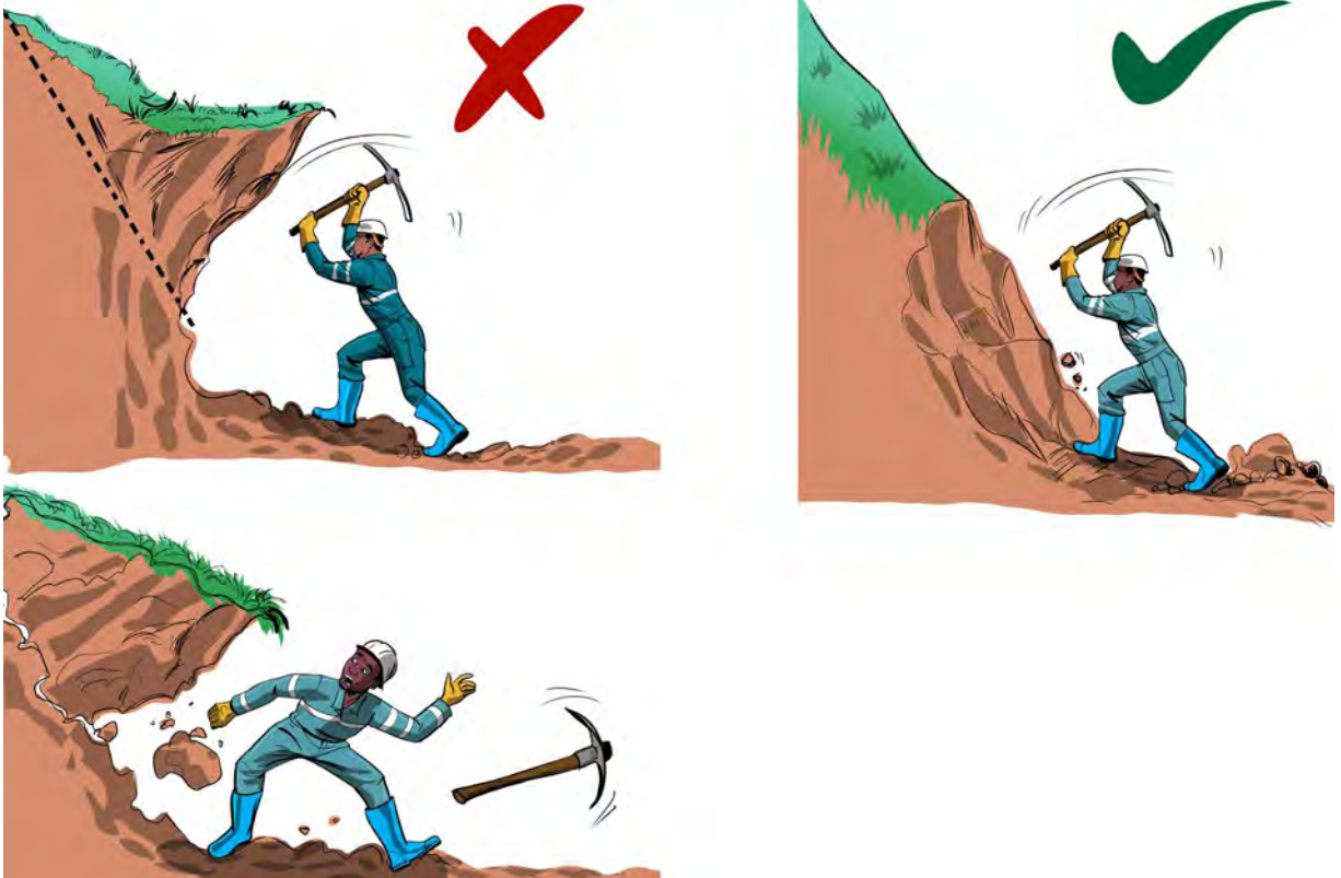
Image 8: To prevent accidents mining needs to be done correctly without leaving steep walls or undercutting.
