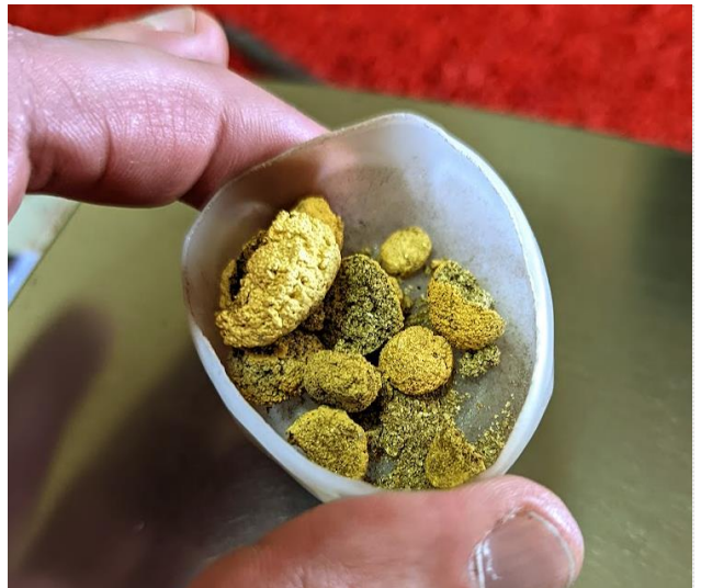
Sponge gold produced with mercury from manual operations, November 2022, Wau, PNG
