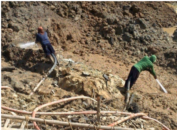
Guyanese alluvial miners using hydraulic jets to pump gold bearing sediment through a sluice, create a concentrate, apply mercury, and produce the gold. | Kevin Telmer
