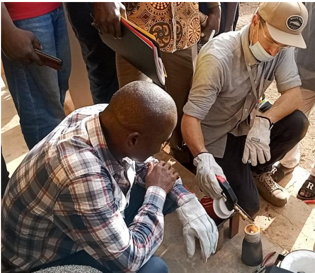
Demonstration of the ‘cupellation method’ in Keniéba
