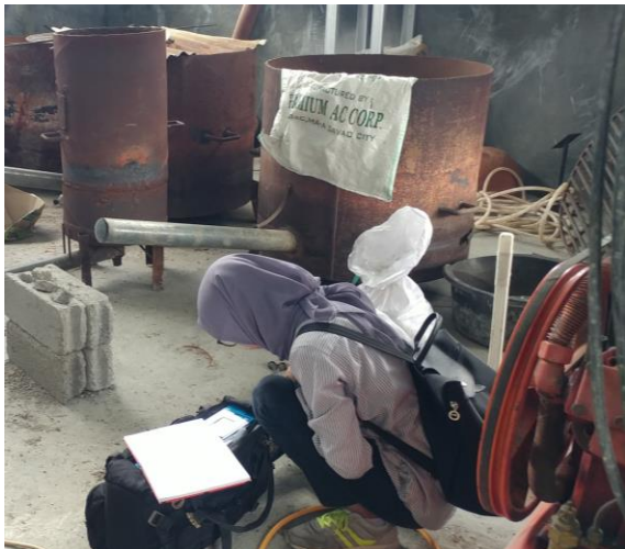
Mercury air sampling with Lumex Portable Mercury Analyzer in ASGM processing area.
