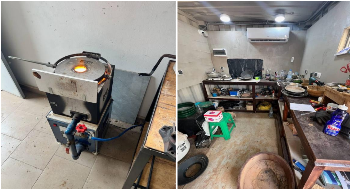
GoldFinX propane gold smelting furnace (left), 40' shipping container workbench in the gold room (right).
