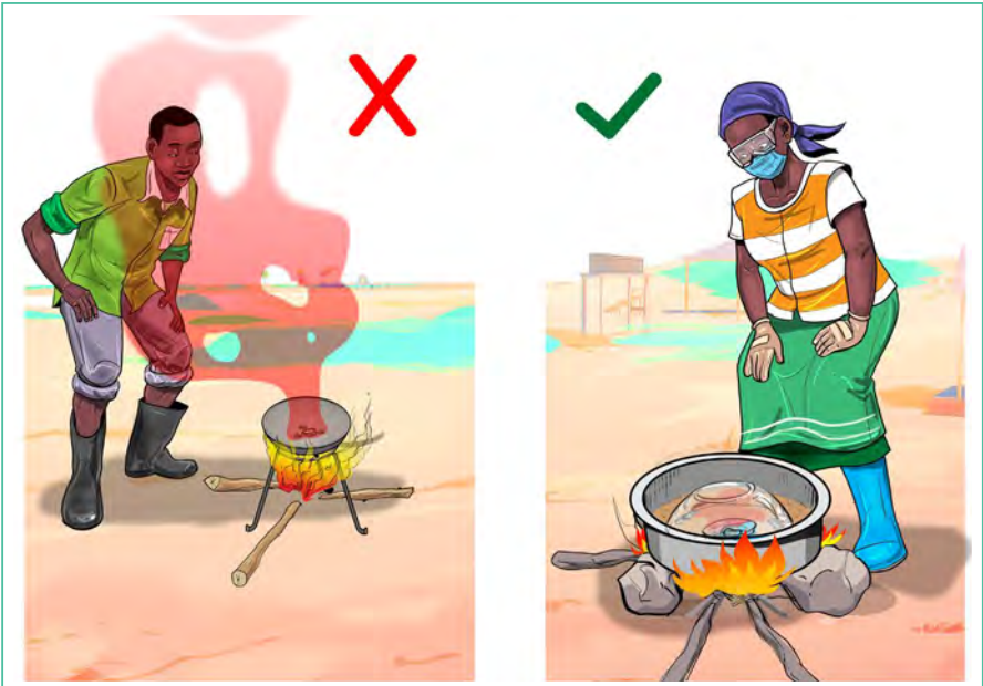
Image 6 : Worst practice is open burning of amalgam. Use a retort.
