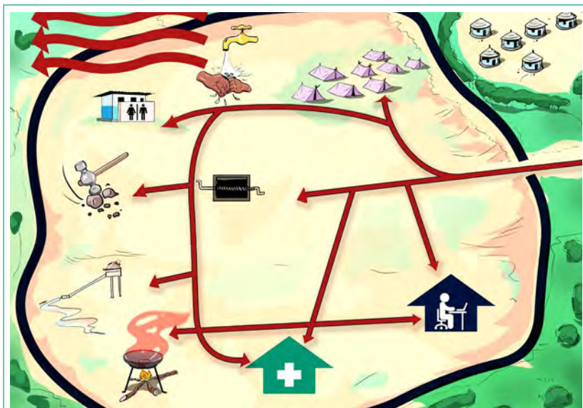
Image 7 : Organize a mine site into different work zones with separate areas for different tasks such as extraction, processing, or burning amalgam.
