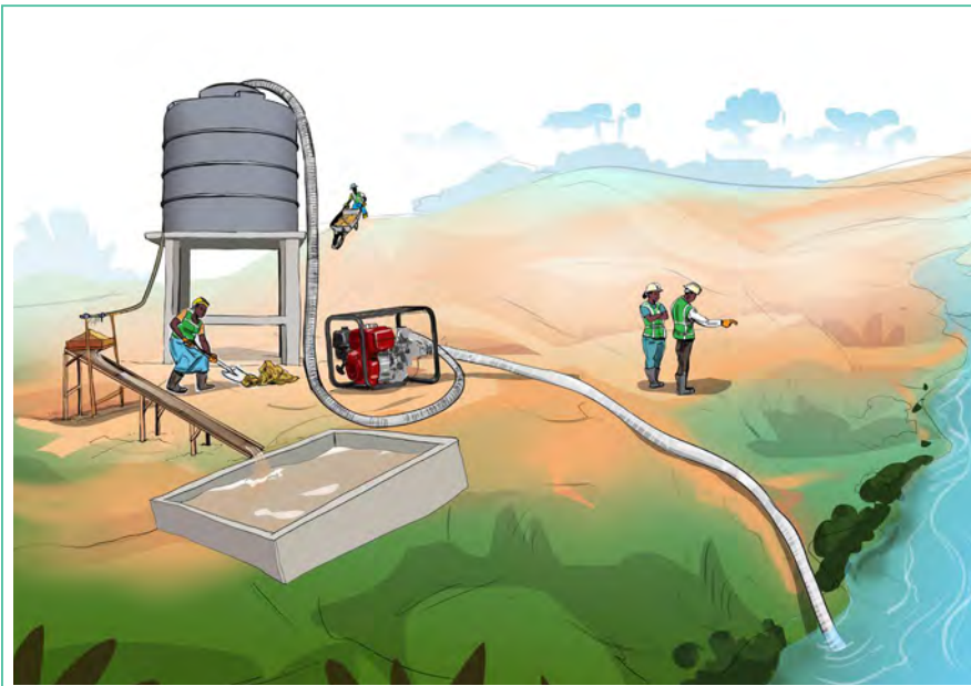
Image 31: Motor pump supplies process water for sluicing.
