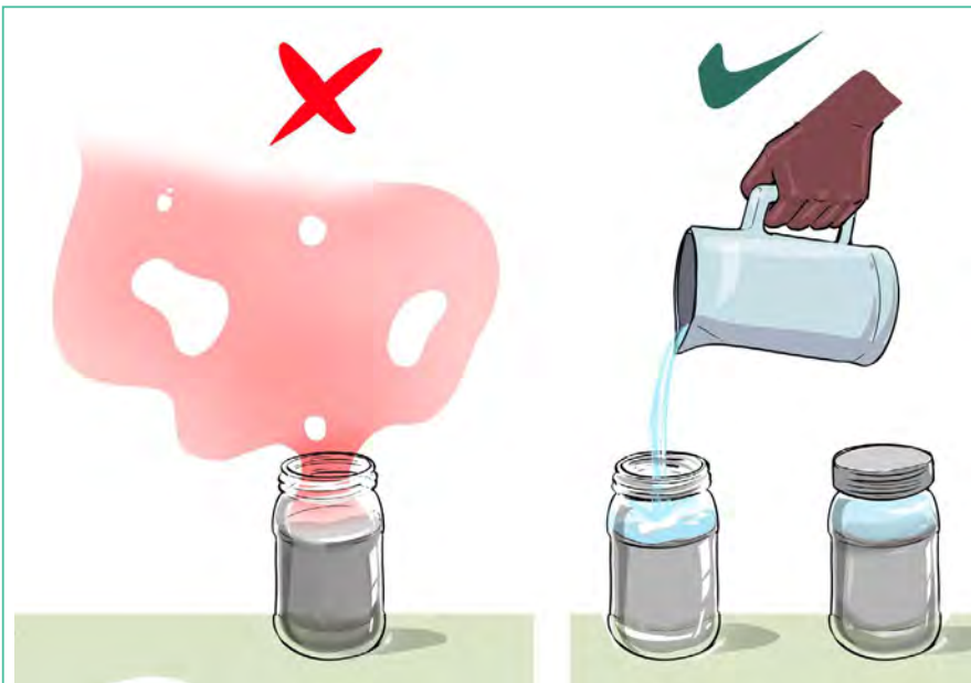
Image 14 : Mercury should be stored in closed airtight containers covered with a centimetre of water.
