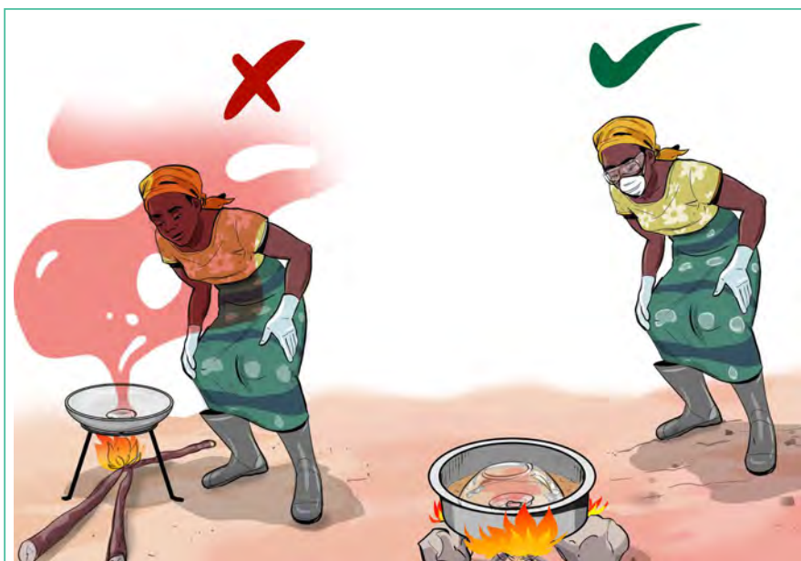
Image 2: Use of mercury in gold extraction such as open burning of amalgam leads to release of vapours.
