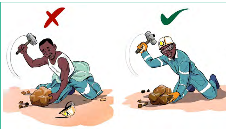
Image 9 : Train miners on the correct way to wear, use, and maintain their PPE.
