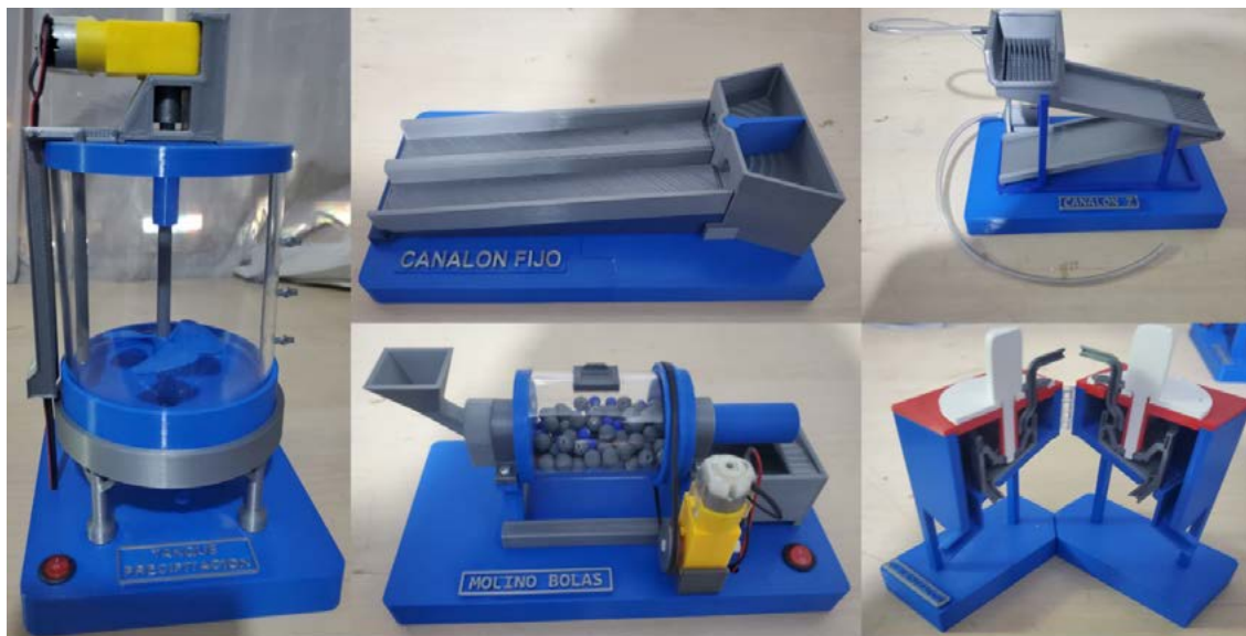
Figure 6: 3D equipment for training small-scale miners as part of planetGOLD Colombia's "I know my plant" process (agitator tank, fixed chute, mobile chute, ball mill, centrifugal concentrator)
