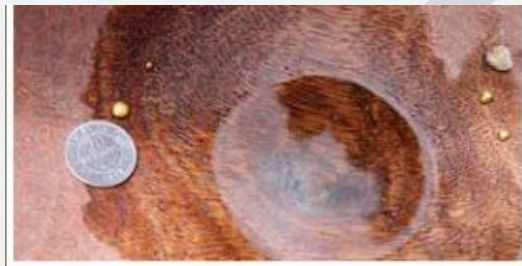
Fig., 33. Results of competition showing gold recovered using borax smelting and amalgamation.
