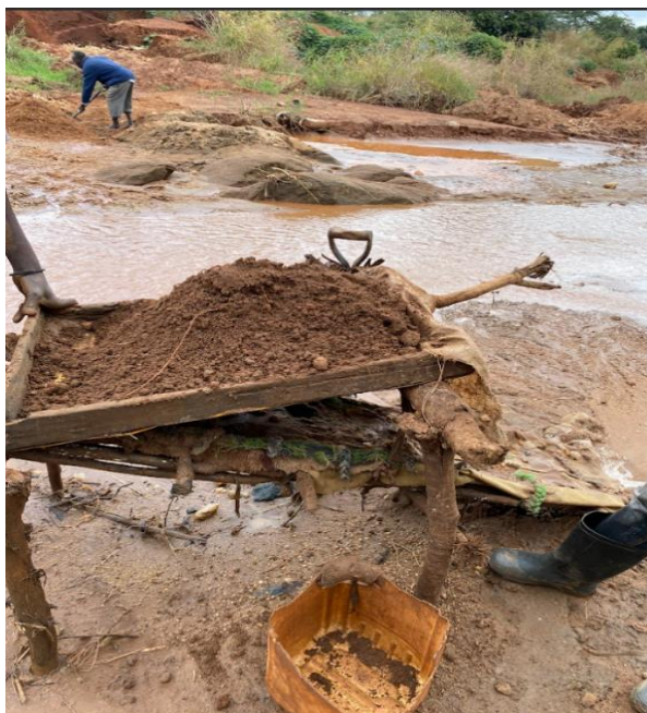
Figure 41: Artisanal tools used for panning gold in Chitumba (Vubwi District)
