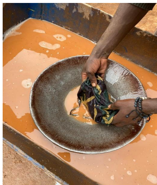
Figure 56: Miner handling Mercury Amalgam without any PPE
