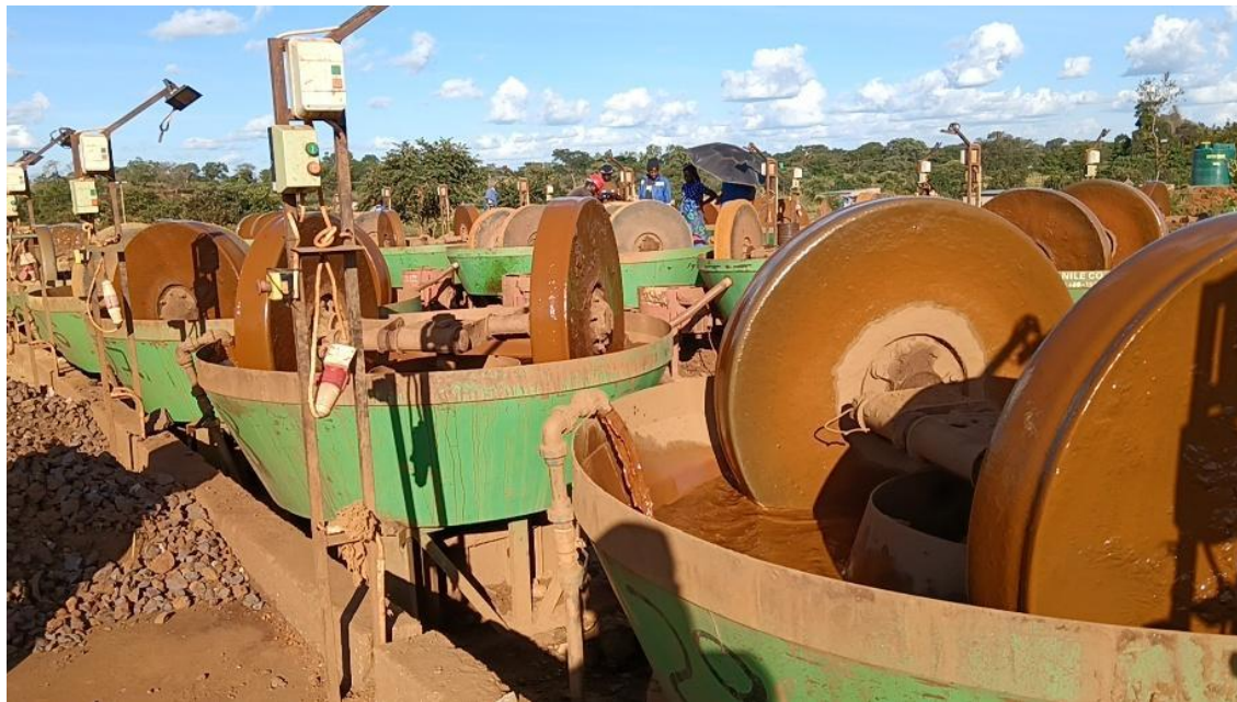
Figure 39: Wet pan processing Plant for Gold in Mumbwa's Luili/Matapa site
