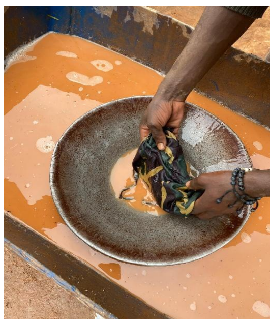
Figure 56: Miner handling Mercury Amalgam without any PPE
