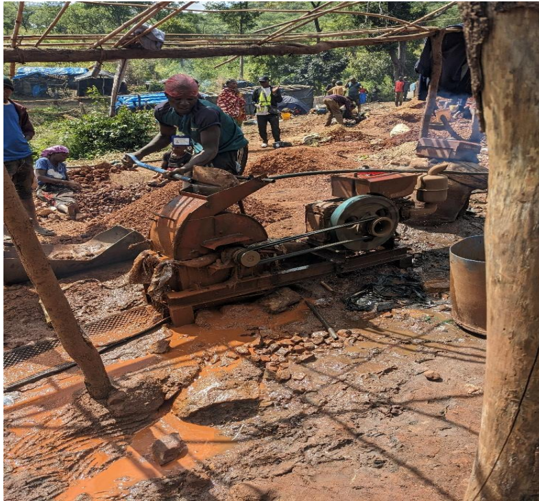
Figure 40: Hammer Mill used for gold processing in Sasare mine
