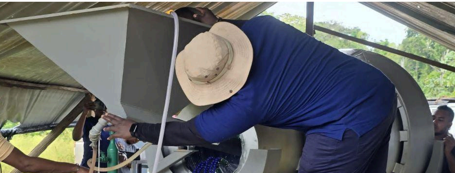
AGC staff demonstrate how to use a helicoidal machine to extract gold without using mercury. Photo by AGC.
