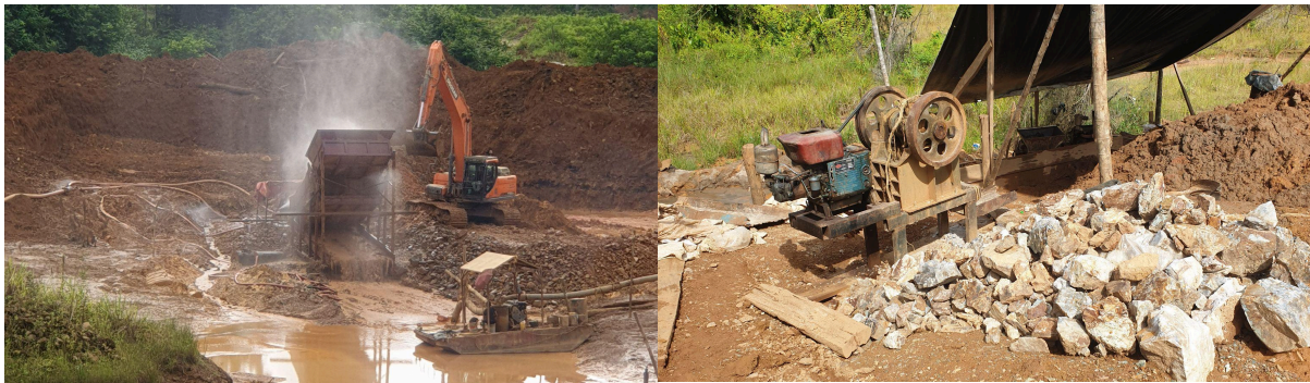
Left to right: A backhoe excavates soil and feeds it into a sluice box for gold recovery in Guyana. A crushing machine processes gold ore to extract valuable minerals. Photos by AGC
